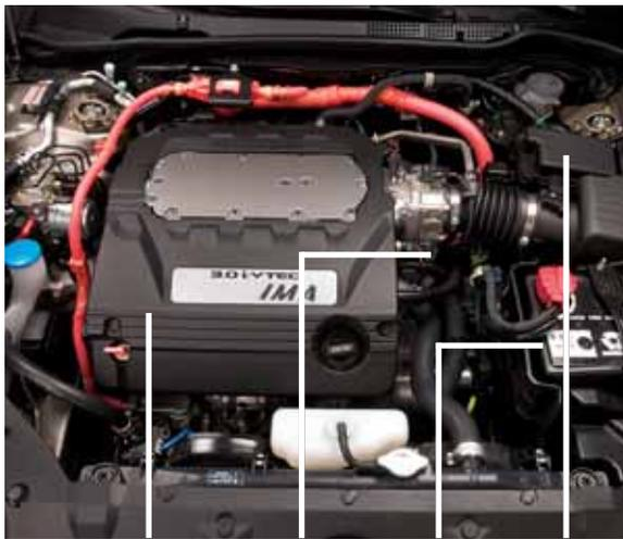
Engine      Motor      12-Volt Battery      Underhood Fuse Box
