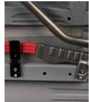
*Thermal shield near hot exhaust*
