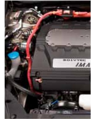
*High-Voltage Cable to Accord AC Compressor*
