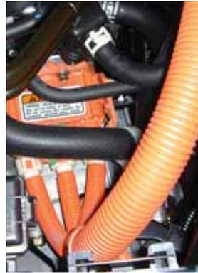
*High-Voltage Cable Connection to Motor*
