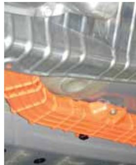
*Electrical shield bolted to undercarriage*
