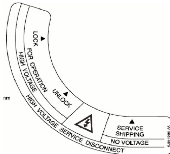
**WARNING – Removing the High Voltage Service Disconnect Switch – disconnects high voltage from the vehicle. The individual cells inside the battery pack will still be charged. Do not cut into the high voltage battery case or penetrate the batteries in any way.**
