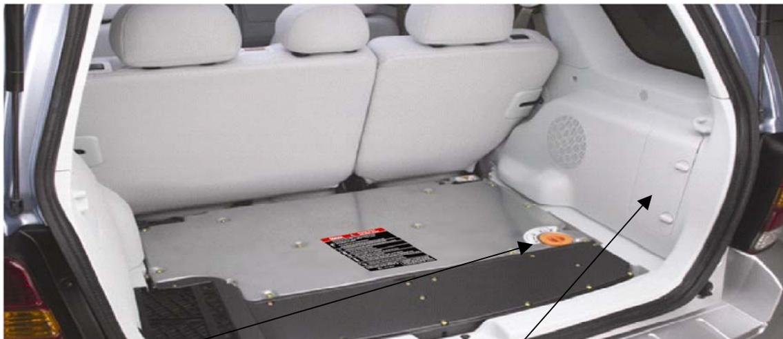
High Voltage Service Disconnect Switch panel
