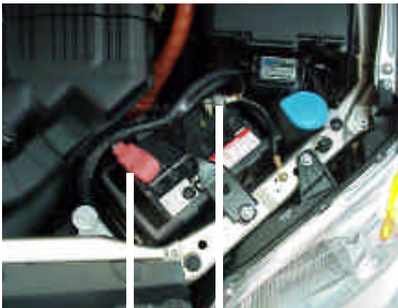
Positive Cable Negative Cable
